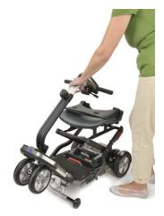
3. Ensure your scooter is locked in the unfolded position by pulling the seat away from the floor pan with one hand and pushing the tiller away from the seat with the other until you hear a click and feel your scooter lock into this position. Once your scooter is locked in position you will no longer be able to move the tiller towards and away from the seat so use this as a simple test to find out if your scooter is locked in the unfolded position.
