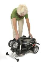
Once folded you can then lift your scooter using the handle at the rear and stand it on its front wheels to move around in the folded position.
