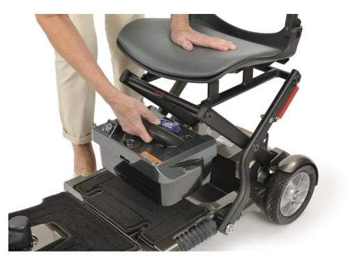
To remove the battery pack first ensure the pack is unlocked by inserting the key into the pack and turning it 90° anti clockwise to the unlock position. Then simply lift the pack up away from the base of the scooter and the seat using the handle provided.
