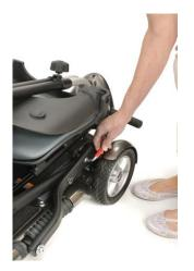
2. Pull the tiller away from the floor pan until the front wheels of your scooter touch the floor.
