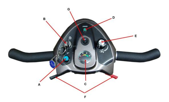
A. Horn – press the horn button to sound your horn.
